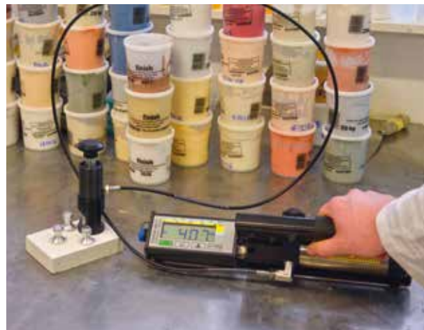
Pull-off adhesion test
