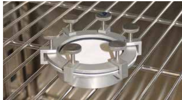
Measurement of breathability in a climatic chamber
